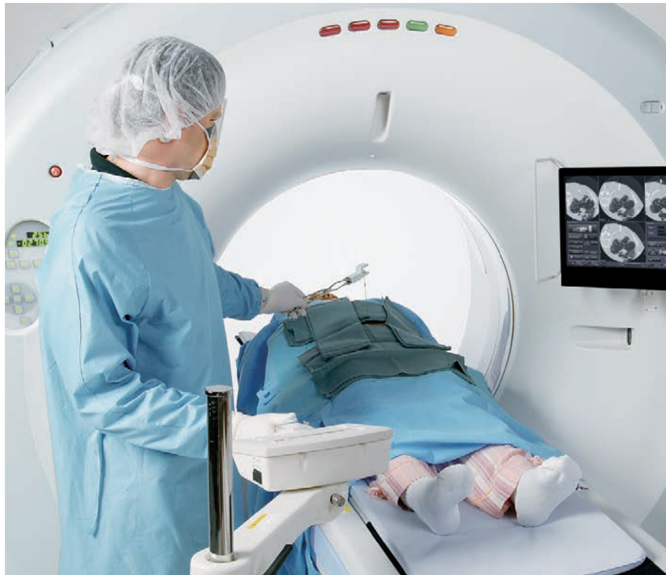
90 cm opening allows unprecedented access to the patient. Specialized needle holder supplied with SUREFluoro provides additional protection to operator without affecting image quality.
